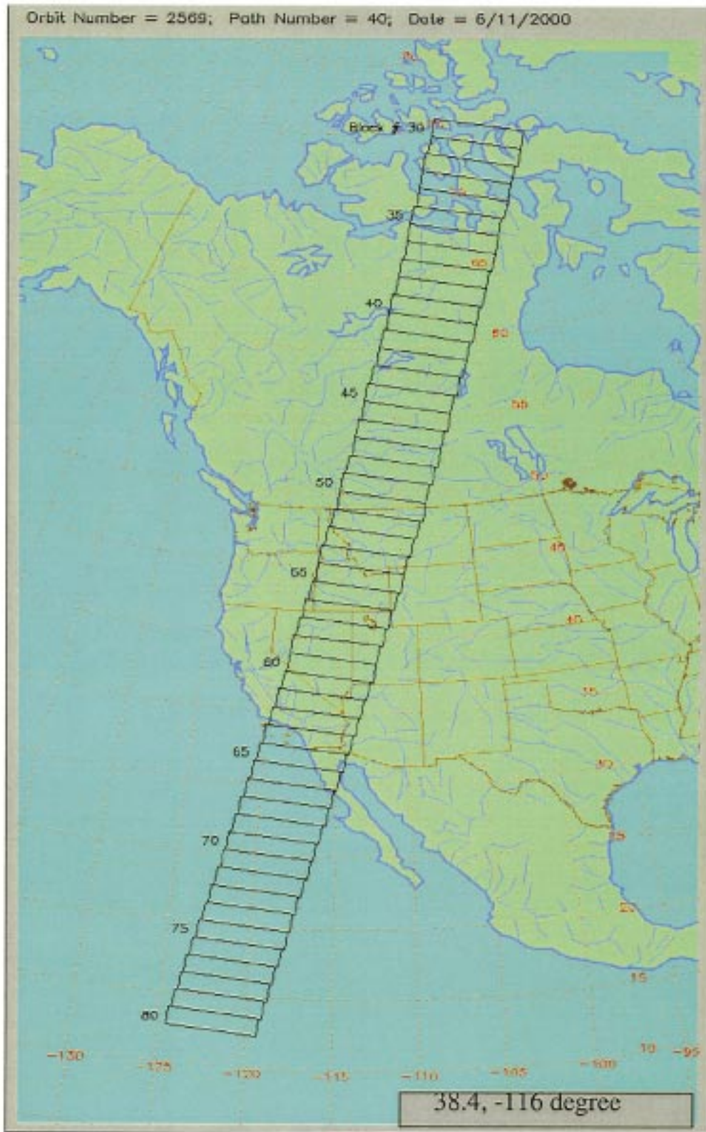
Fig. 1. Illustration of MISR footprints in path 40, orbit 2569 on June 11, 2000. Each path is divided in 180 blocks. Block 60 contains the data measured over Lunar Lake, NV, and is used in the analyses described in this paper.
