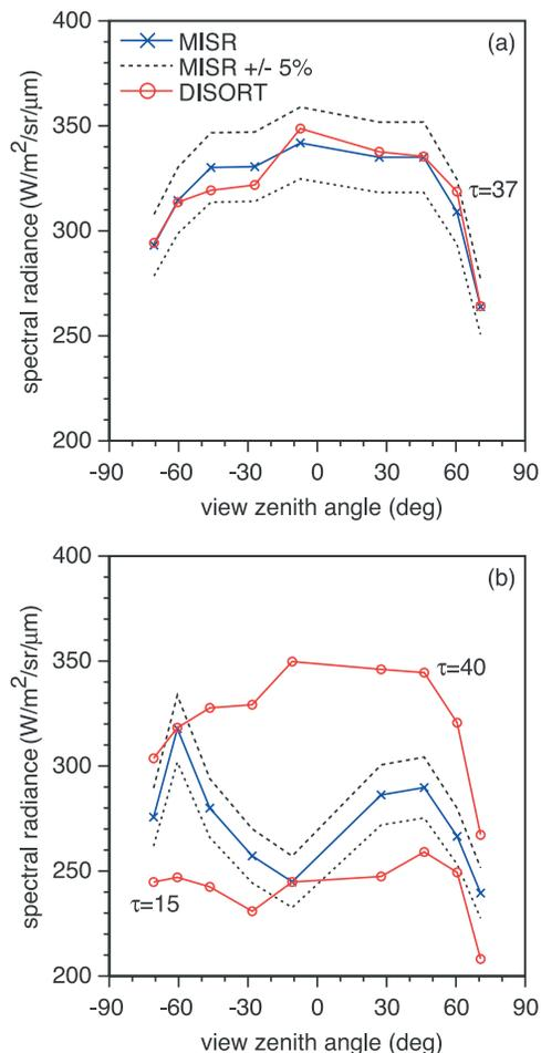
**Figure 1.** Comparison of measured and plane-parallel angular reflectances at a resolution of 275 m. (a) Cloud passes the angular test. (b) Cloud fails the angular test. Both examples are from block 118 (centered at 34°S, 113°E) of orbit 6156. The solar zenith angle is 33° and the measurements are approximately in the 40°/220° azimuthal plane. Data points with negative (positive) view zenith angles are in the forward (backward) scattering direction.
