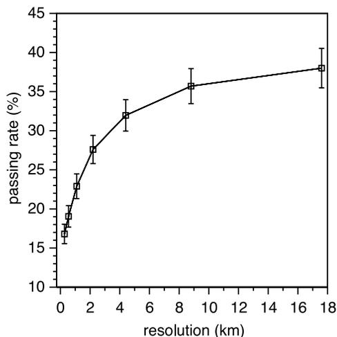
**Figure 2.** Angular test passing rate vs. pixel resolution for  $R_e = 8 \mu\text{m}$ . Error bars correspond to the standard error in the mean.
