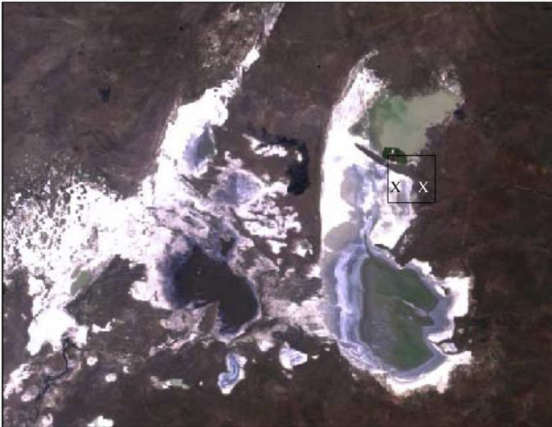
Fig. 1. MISR image of Sua Pan, Botswana (20.6° S, 26.1° E), on the clear day of August 27. The image is an RGB composite from the nadir camera, at 275-m resolution. The rectangular box shown in this figure defines the ground campaign site. The “X” marks the locations of the ground and airborne measurements used in the analyses. MISR image of Sua Pan on September 3 (not shown here) shows heavy haze due to smoke from biomass fires that were present near Sua Pan.
