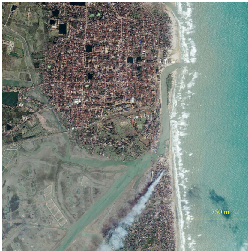
Fig. 5. IKONOS 1 m color image of Nagapattinam, India obtained on 29 December 2004, 3 days after the tsunami. In the northern part of the image, damage to buildings is evident along the coast. The scale in the lower right shows 750 m, which was the estimated distance inland the tsunami waves penetrated along a transect just to the north of the cooking oil tanks that can be seen as the group of white circles on the beach in the north-central part of the image (Ramanamurthy et al., 2005). The southern portion of the image shows the Vedaranyam Canal. The tsunami waves penetrated more than 2 km inland along this waterway and much of the adjacent land appears to be covered in silt. Plumes of smoke in the lower center of the image are most likely from burning debris. Image courtesy of Space Imaging.
